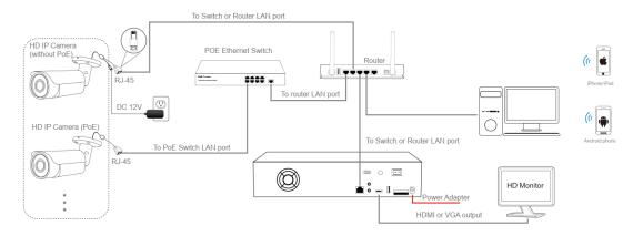
Figure 2: Working With PoE switch and NVR
