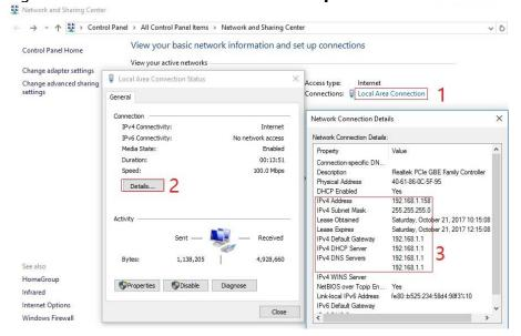
If the camera is installed to work with the local switch or router directly, the camera IP range should be 192.168.1.x (x=2-254). To void IP conflict, you should test and select an unoccupied IP like this:
