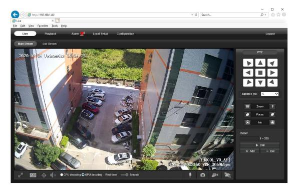
**Note:** Only the **Motorized Auto Focus** cameras can **Zoom In** and **Zoom Out.** Keeping pressing on live video and dragging for **Digital Zoom**.
