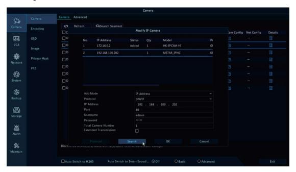
**Note:** Some of the PoE NVR supports **Plug & play**, which allows you to get video without manually search and add. if **Plug & play** feature is not available or not compatible, please follow the NVR manual steps and select **ONVIF** protocol as the paring protocol. *(camera default password: 123456)*
